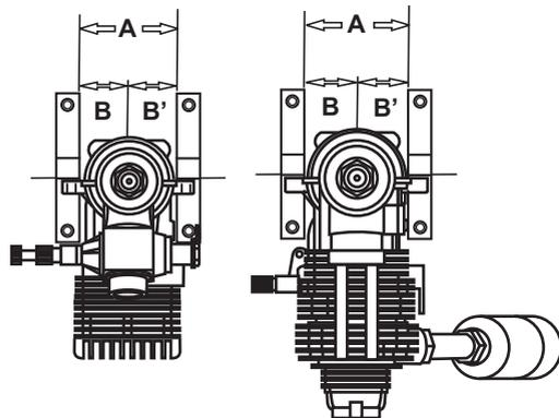
! Align the mark on both engine mount beams with the mark on the fuselage
