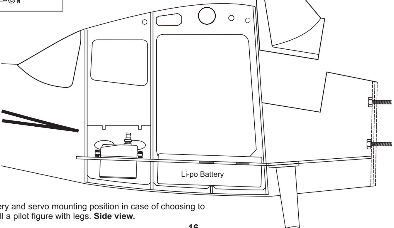
Battery and servo mounting position in case of choosing to install a pilot figure with legs. **Side view.**
