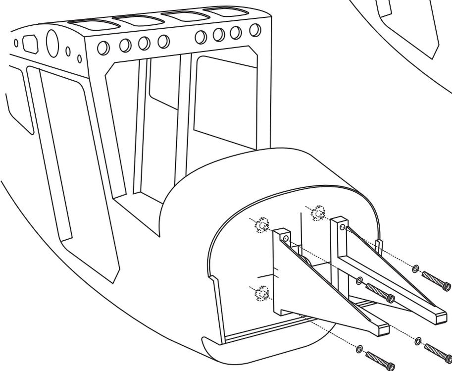
Insert the blind-nut onto each of the four holes make above.
