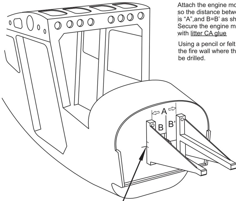
Attach the engine mount beams onto the fire-wall so the distance between of two engine mount beams is "A", and B=B' as show.
