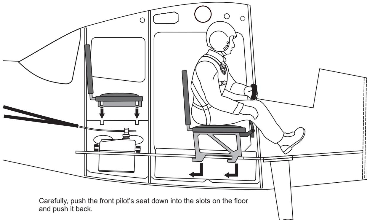
Carefully, push the front pilot's seat down into the slots on the floor and push it back.
