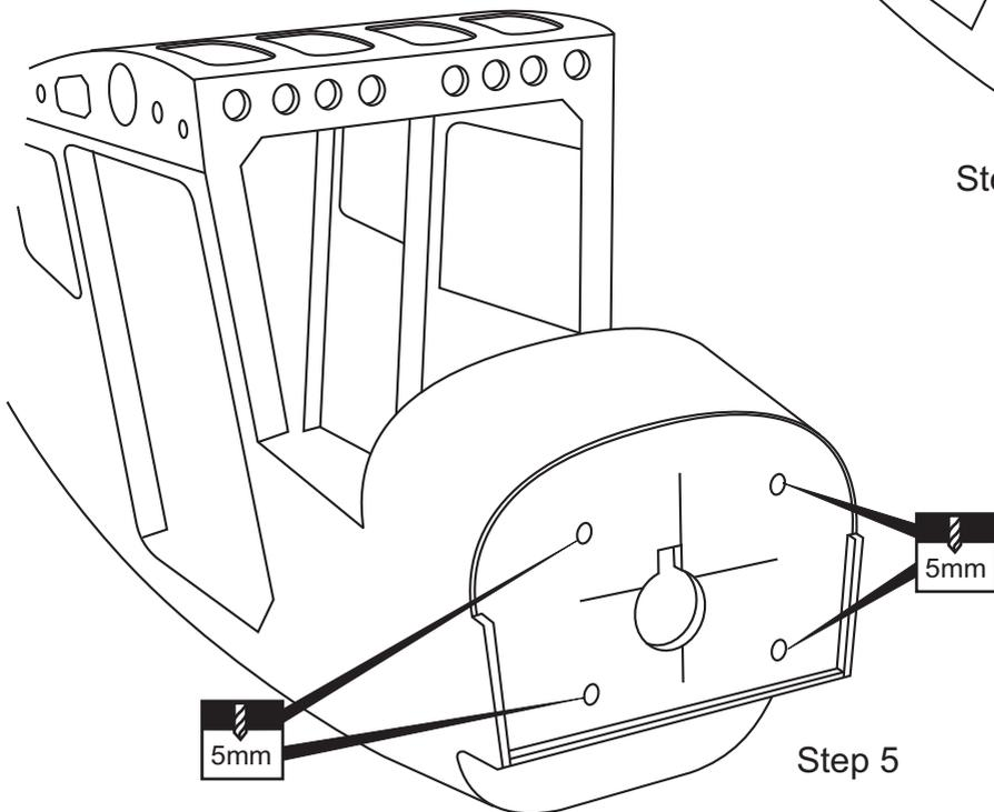
Remove the wooden motor mounting plate and drill a 5mm hole through the fire-wall at each of the four marks marked .
