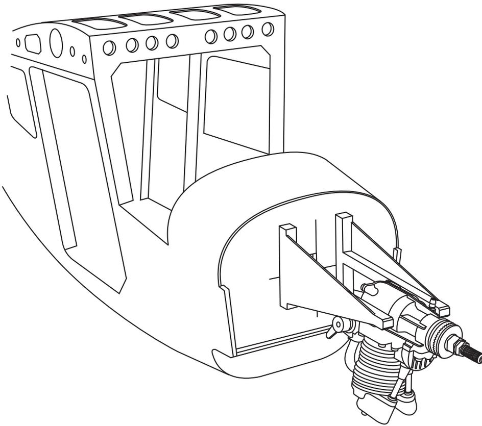
Reposition the engine on the engine mount beams, aligning it with the holes. Secure the engine to the engine mount using four 3x25mm screws.
