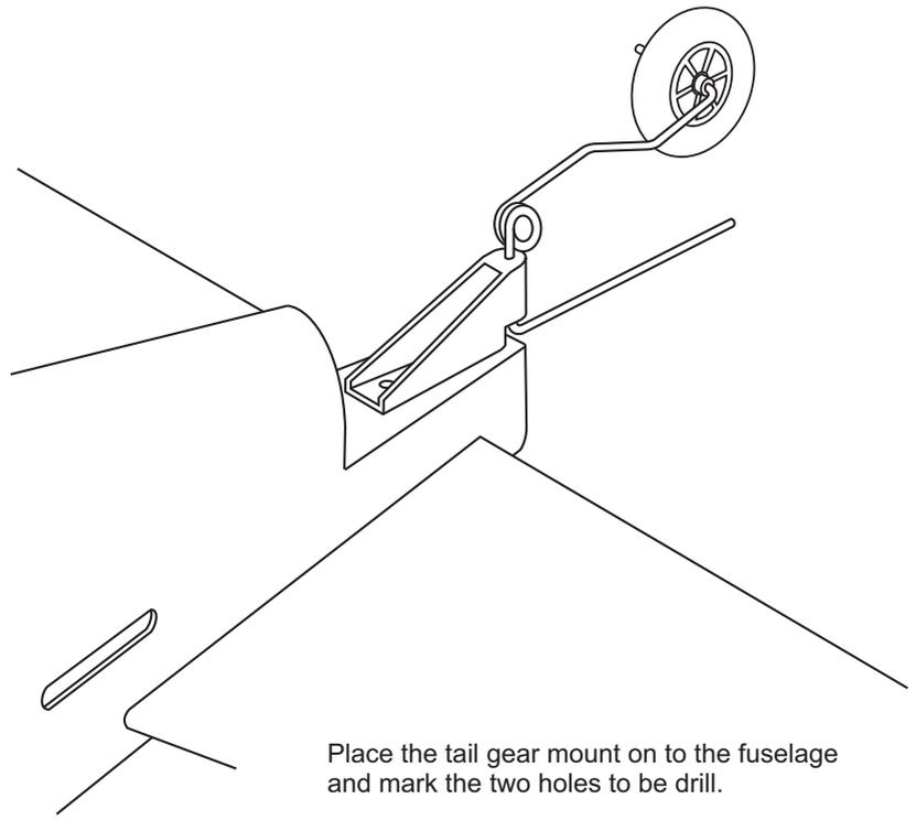
Place the tail gear mount on to the fuselage and mark the two holes to be drill.
