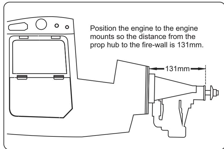
Position the engine to the engine mounts so the distance from the prop hub to the fire-wall is 131mm.
