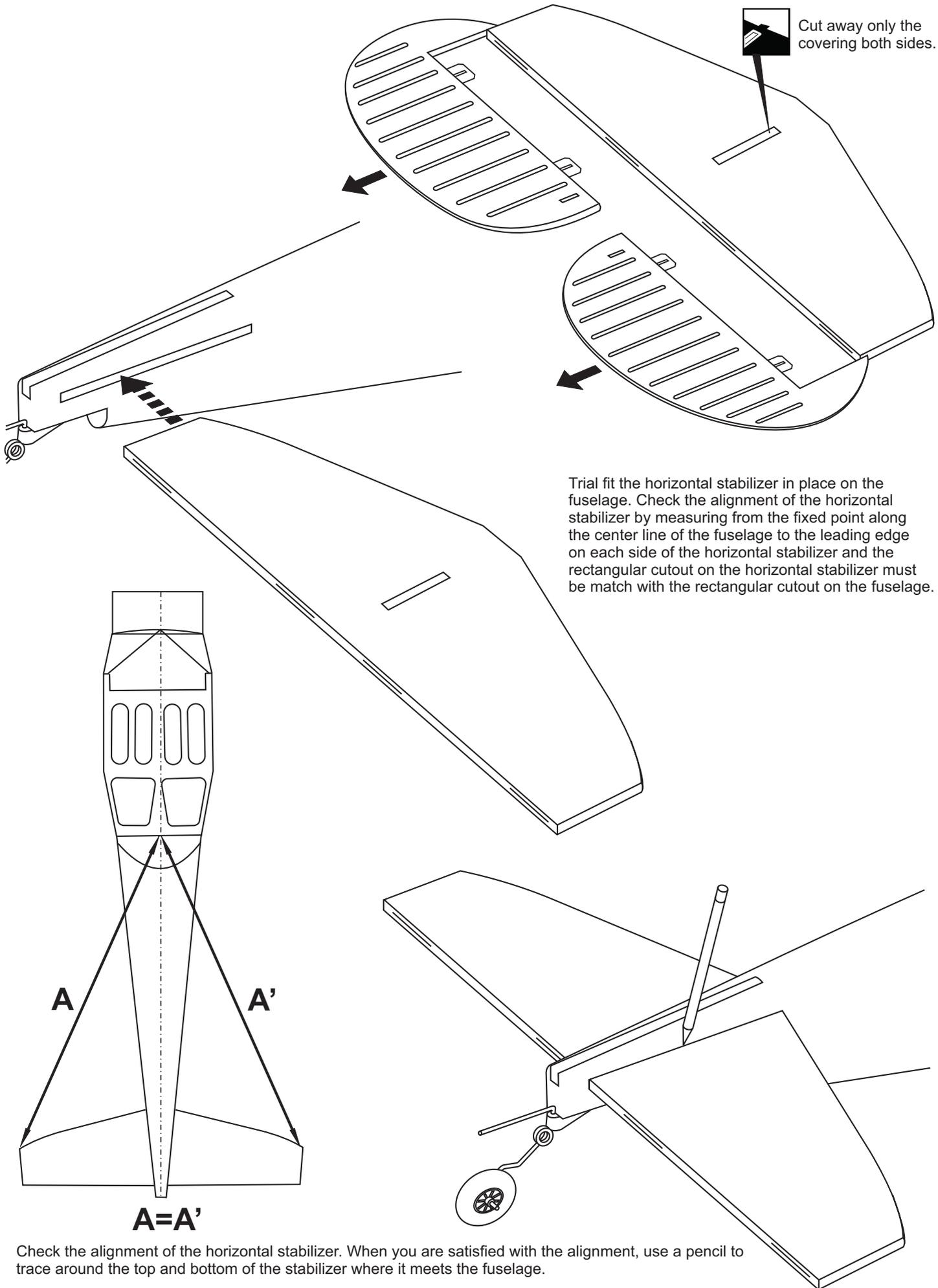
Remove the horizontal stabilizer from the fuselage. Using a straight edge and a sharp hobby knife, carefully cut away the covering **inside the lines** which were marked above. Be cautious **not to cut into the wood**-this will weaken the structure.
