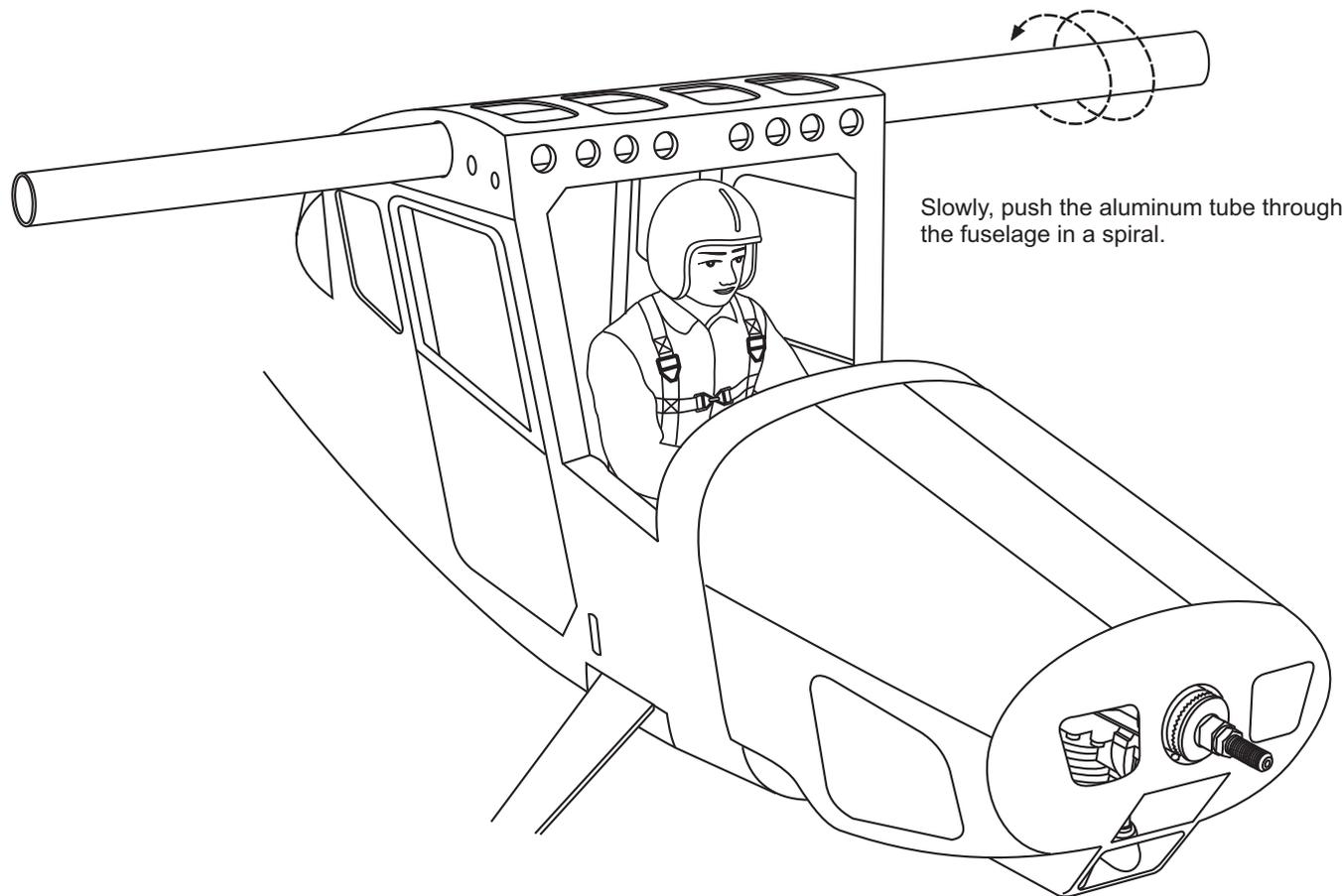
Slowly, push the aluminum tube through the fuselage in a spiral.
