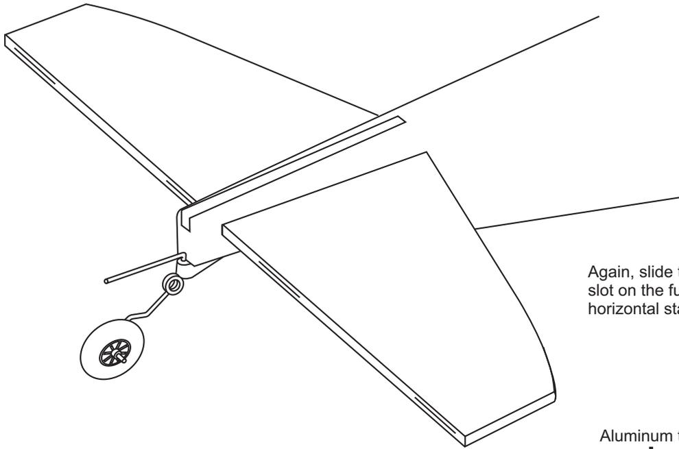
Again, slide the horizontal stabilizer into the slot on the fuselage. Check the alignment of the horizontal stabilizer.
