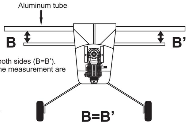
The distance must be equal on both sides ( $B=B'$ ). If not, adjust the stabilizer until the measurements are the same.
