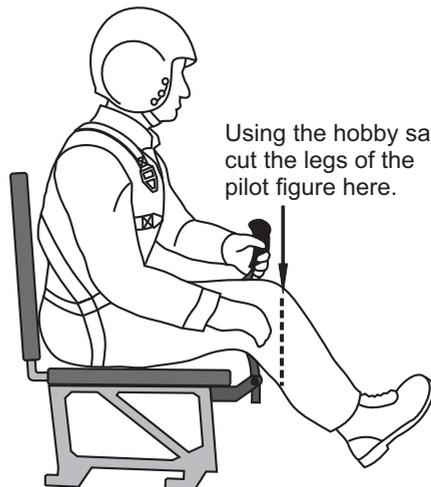
Using the hobby saw, cut the legs of the pilot figure here.
