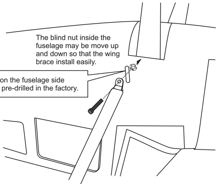
The blind nut inside the fuselage may be move up and down so that the wing brace install easily.
