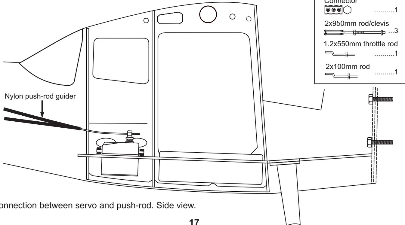
Connection between servo and push-rod. Side view.
