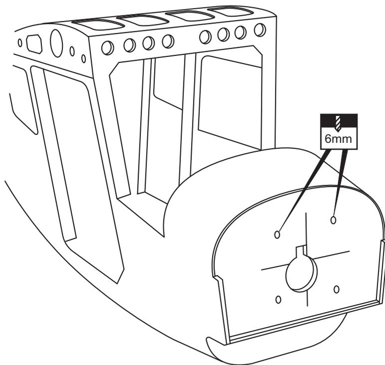
Carefully remove the engine mount beams and drill a 6mm hole through the fire-wall at each of the four marks made above.
