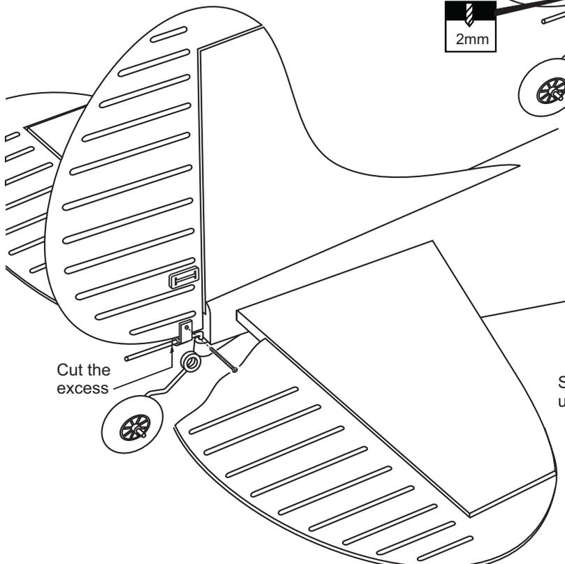
Secure the tail gear control horn in place using 2x10mm screw and nut.
