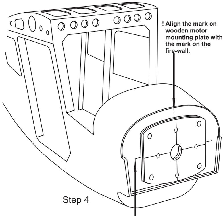
! Align the mark on wooden motor mounting plate with the mark on the fire-wall.
