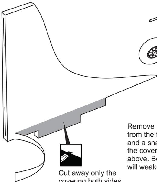
Remove the vertical stabilizer from the fuselage. Using a straight edge and a sharp hobby knife, carefully cut away the covering **inside the lines** which were marked above. Be cautious **not to cut into the wood**-this will weaken the structure.
