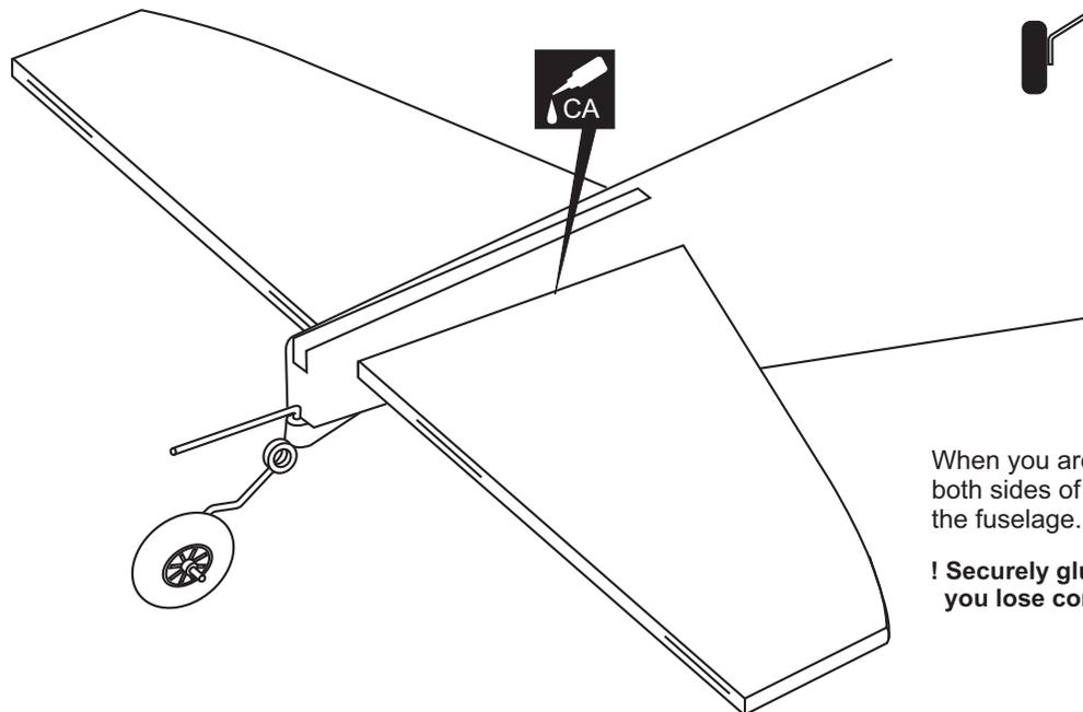
When you are satisfied with the alignment, glue the both sides of the horizontal stabilizer where it meets the fuselage.
