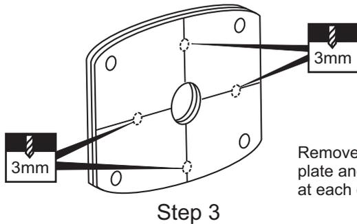
Remove the aluminum motor mounting plate and drill a 3mm hole through the plywood at each of the four marks marked .
