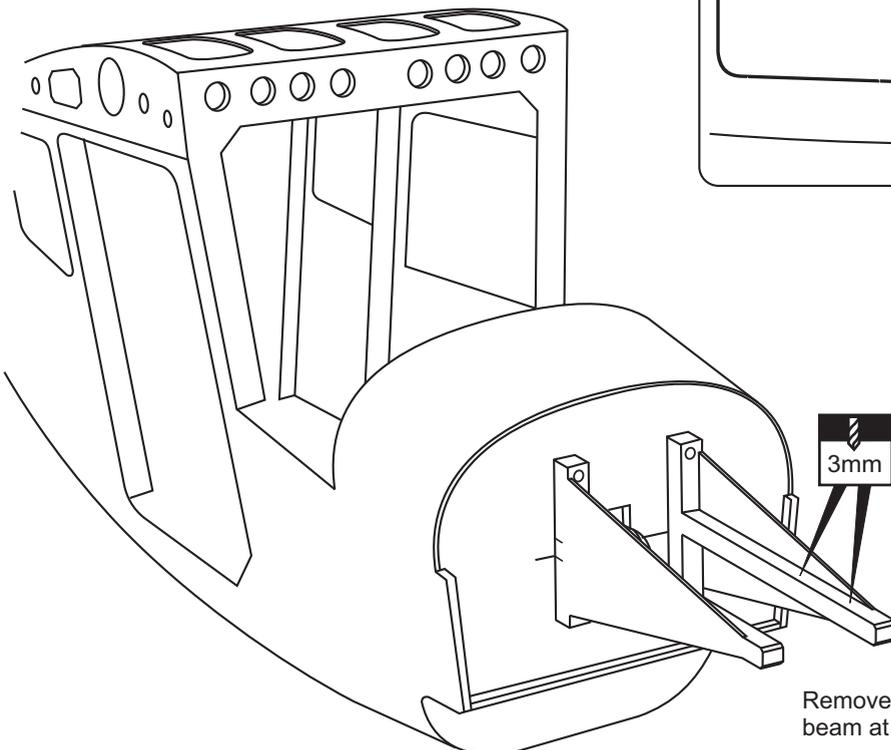
Remove the engine and drill a 3mm holes through the beam at each of the four marks made above.
