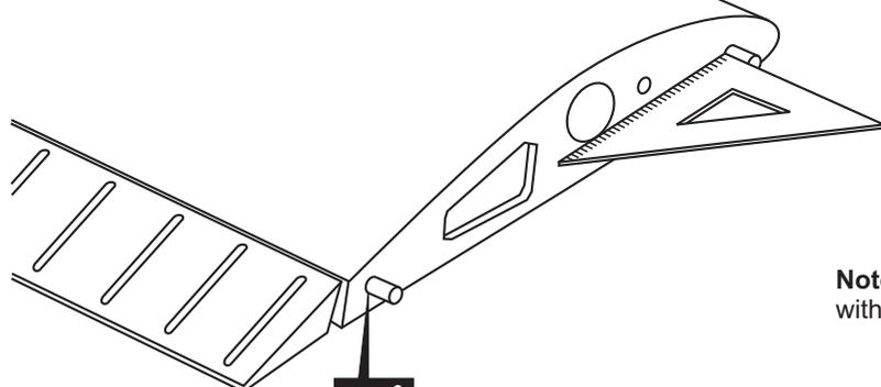
**Note:** The wooden dowels must be perpendicular with the root rib.
