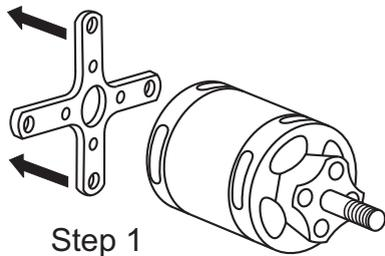
Using a aluminum motor mounting plate as a template, mark the plywood motor mounting plate where the four holes are to be drilled.
