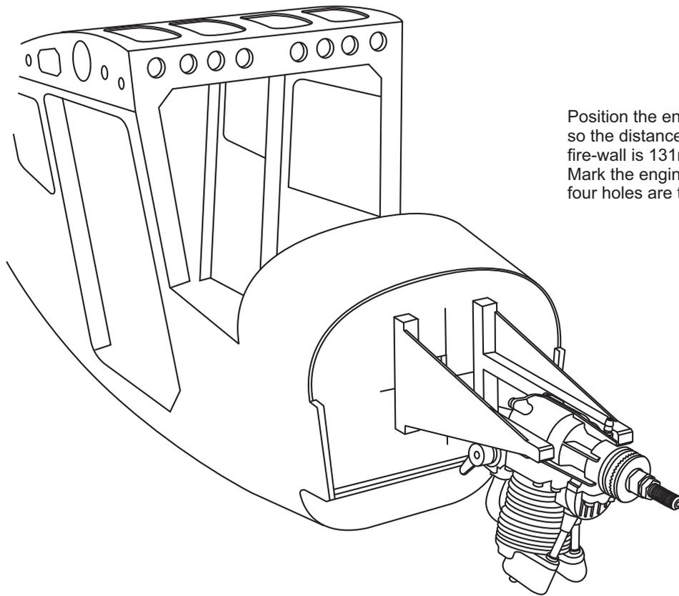
Position the engine to the engine mounts so the distance from the prop hub to the fire-wall is 131mm.
