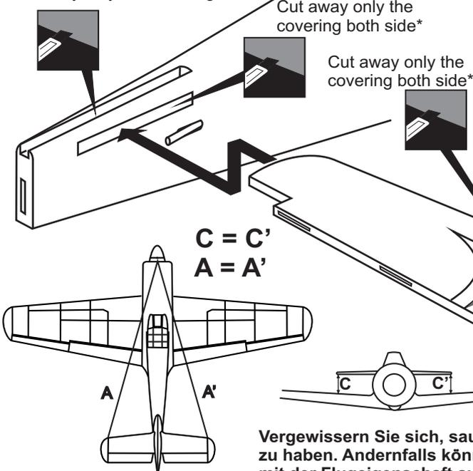
1-Trial fit the horizontal stabilizer in place . Check the alignment of the horizontal stabilizer. When you are satisfied with the alignment, use a pencil to trace around the top and bottom of the stabilizer where it meets the fuselage.
