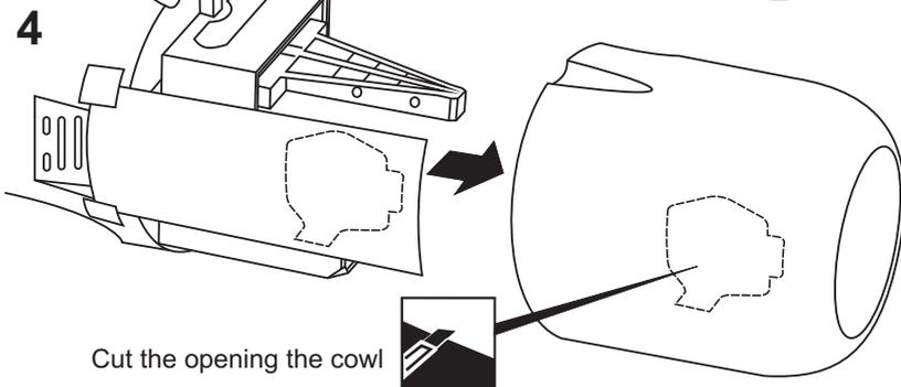
Remove the cowl from the fuselage and carefully cut the opening for the engine head through as marked above. Do the same way with the hole for needle-valve.
