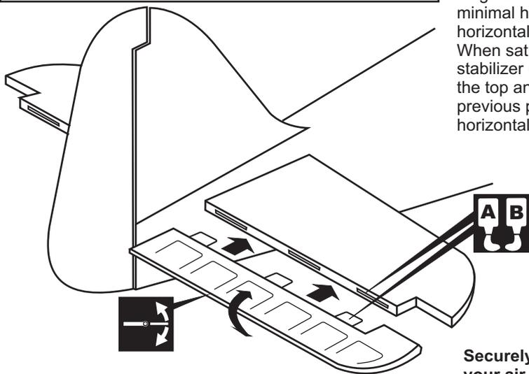
Apply a thin layer of machine oil or petroleum jelly to only the pivot point of the hinges on the elevator, then push the elevator and its hinges into the hinge slots in the trailing edge of the horizontal stabilizer. There should be a minimal hinge gap and the end of the elevator should not rub against the horizontal stabilizer.
