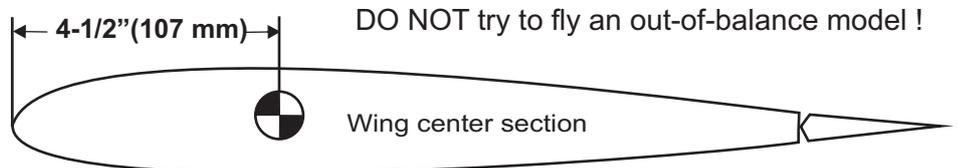
To get the correct C.G., Several strips of lead weight were required in the nose of this model .
