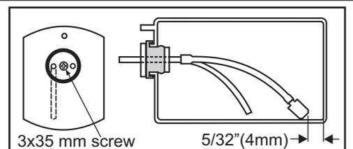
After confirming the direction . Insert and tighten the screw.
