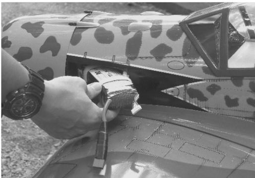
Again, put the magnetic battery hatch in place.
