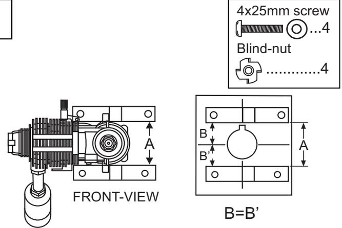
Attach the engine mount beams onto the fire-wall so the distance between of two engine mount beams is "A".
