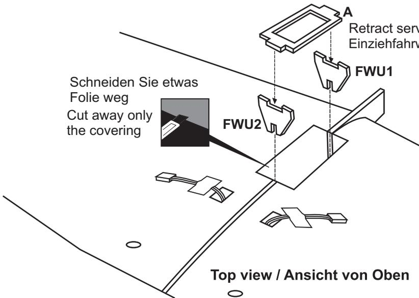
Retract servo mount (plywood A,B,C)
