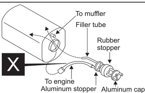
Push the fuel tank forward until there are no gaps between the tank and firewall.
