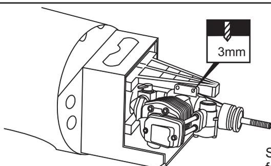
Secure the engine with four 3x20mm screw
