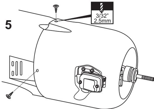
Reposition the engine onto the engine mount beams and secure it with four 3x25mm screw.
