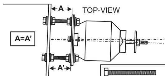
! Engine thrust on balk head is already adjust at factory
