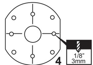
! Align the mark on the plywood motor mount with the center lines on aluminum motor mount.
